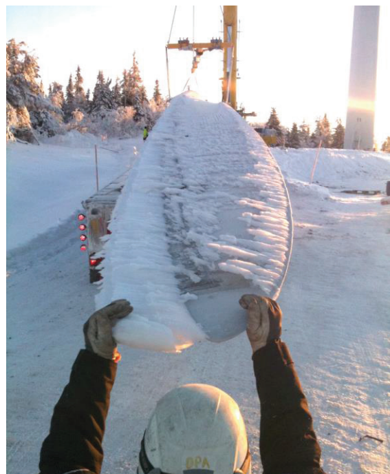
Figure 7-1: An iced-up wind turbine blade. Photo credit: Göran Ronsten
