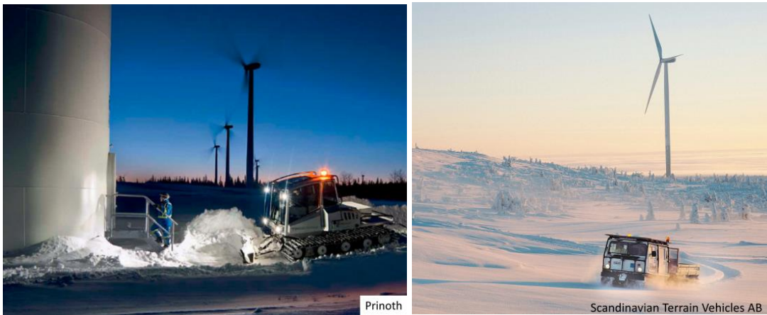
Figure 18: Examples of tracked vehicles (snow cats) used to access wind turbines [232]
