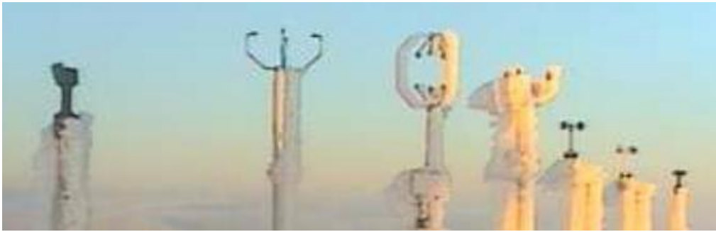
Figure 6. Testing different wind anemometers in severe icing climate (source: [42])
