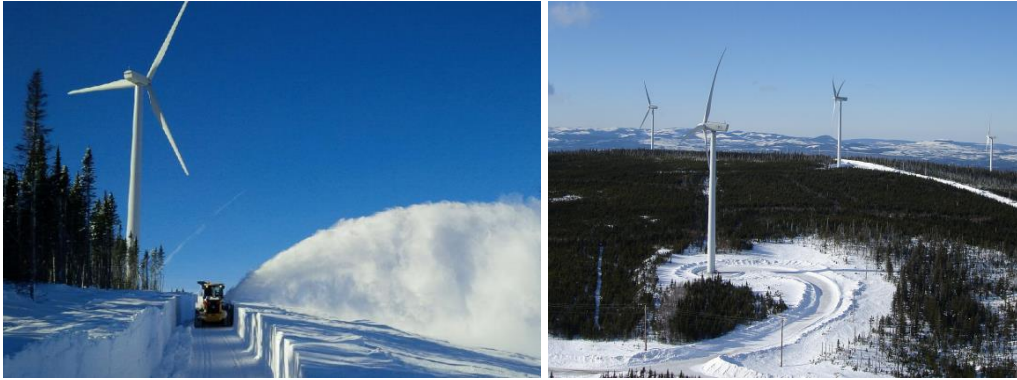
Figure 17: Snow removal allows for easy access to turbines with regular service vehicles but can be very expensive [232]
