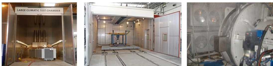
Figure 26: Climate chamber examples for testing electro-mechanical wind turbine systems
