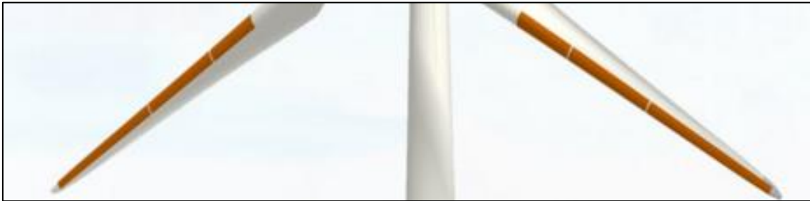
Figure 14: Retrofit electro-thermal ice protection system (source: ADIOS)
