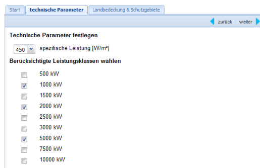
Fig. 4 Exemplary layout of WebGIS application with possibility to manually select the turbines sizes that shall be used for the calculation of the realizable energy yield.
